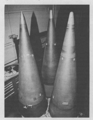
REENTRY TRIO — Three Mk12A reentry vehicles were used in the May 21 operational test. The experimental ultra-high temperature ceramic nose tip, with a sharper point, rode on the RV at left. The other two RVs had standard blunted carbon-carbon nose tips. The photo was taken at Vandenberg prior to launch.
